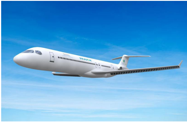
Figure 16. Distributed Propulsion - Illustration of the DRAGON concept [8].
