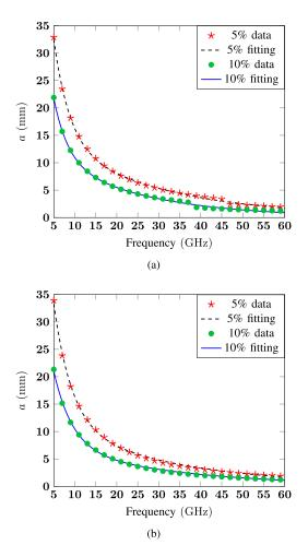
Fig. 3. Curvature radius *a* corresponding to 5% or 10% variations in terms of  $APD_{\text{max}}$  as a function of frequency for (a) TE polarization, and (b) TM polarization.
