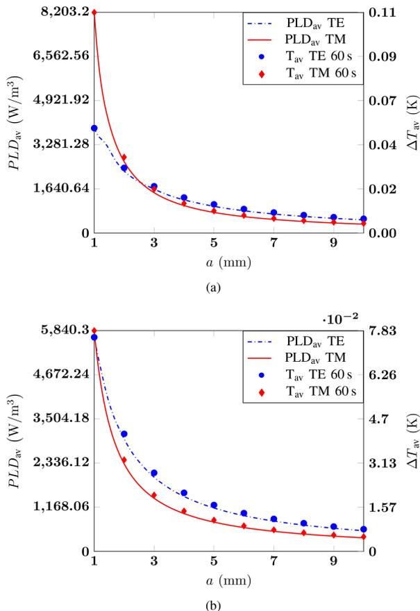
Fig. 5.  $PLD_{av}$  (left axis) and  $\Delta T_{av}$  after a 60 s exposure (right axis) as a function of the curvature radius  $a$  at (a) 26 GHz and (b) 60 GHz.
