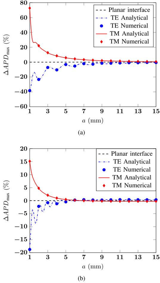
Fig. 2. Variations of the  $APD_{\max}$  as a function of the curvature radius with respect to the planar interface at (a) 26 GHz and (b) 60 GHz.
