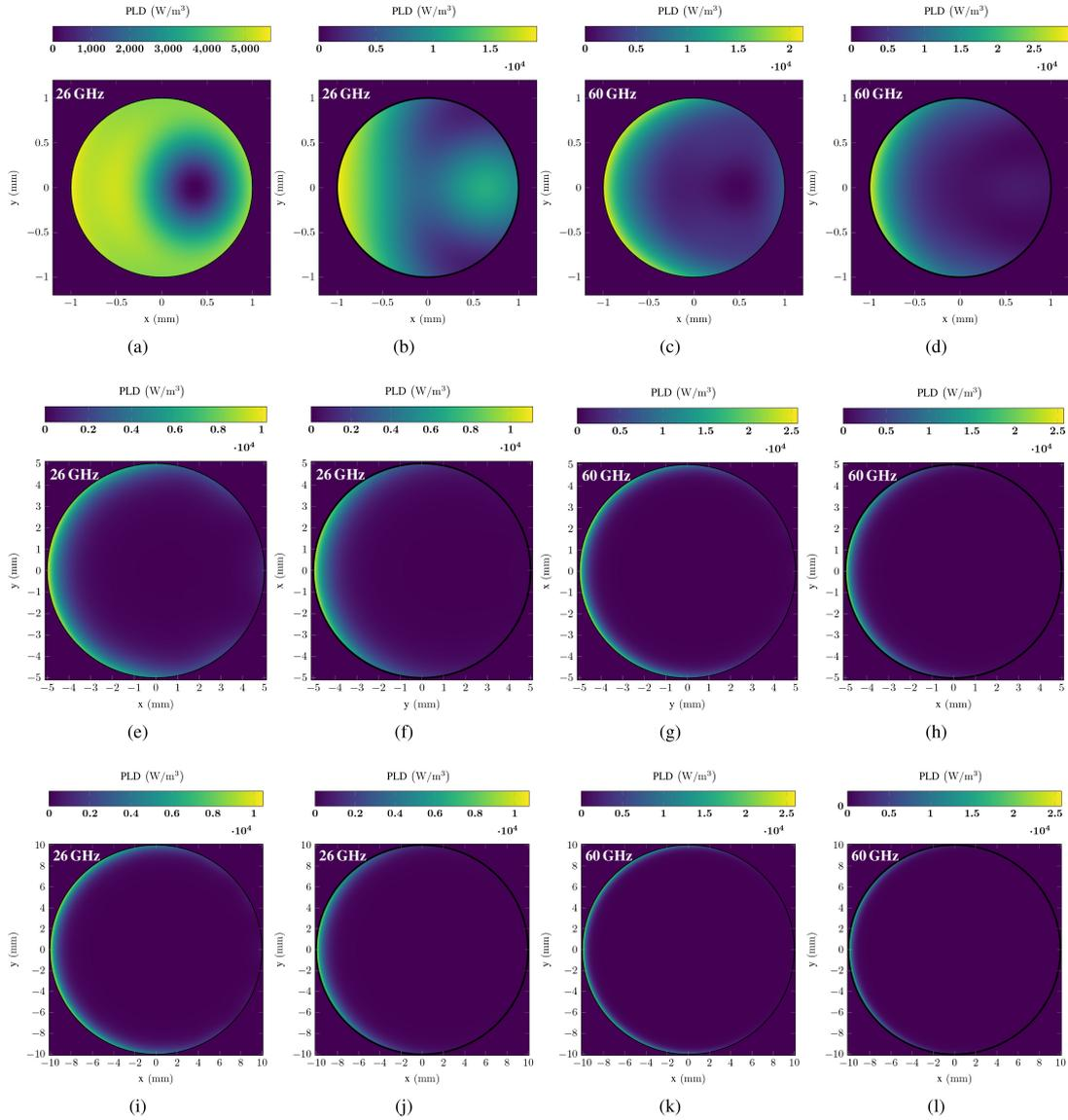
Fig. 4. PLD distribution over the cylinder section for  $a = 1$  mm [(a) TE and (b) TM polarizations at 26 GHz, (c) TE and (d) TM polarizations at 60 GHz],  $a = 5$  mm [(e) TE and (f) TM polarizations at 26 GHz, (g) TE and (h) TM polarizations at 60 GHz], and  $a = 10$  mm [(i) TE and (j) TM polarizations at 26 GHz, (k) TE and (l) TM polarizations at 60 GHz].
