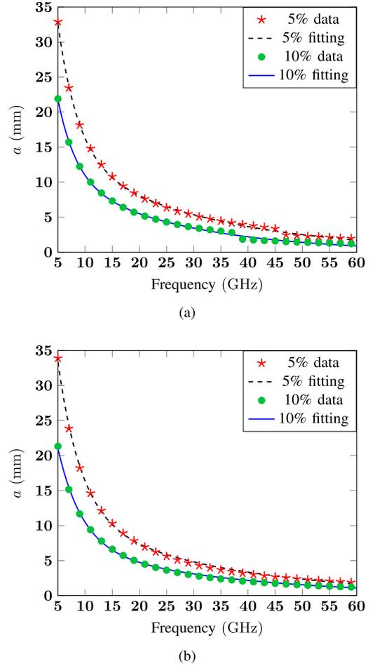
Fig. 3. Curvature radius  $a$  corresponding to 5% or 10% variations in terms of  $APD_{\max}$  as a function of frequency for (a) TE polarization, and (b) TM polarization.
