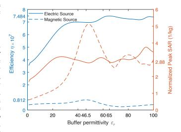
Fig. 3. Efficiency and the peak SAR normalized by the transmitted power as a function of the buffer permittivity for the electric source (continuous line) and magnetic source (dashed line) considering the buffer thickness in which the global maxima are located (d=7 mm for the electric source and d=6 mm for the magnetic source).
