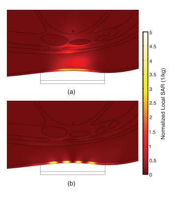
Fig. 4. Surface plot of the local SAR normalized by the transmitted power in the region around the transmitter and receiver for the (a) electric source and (b) magnetic source.
