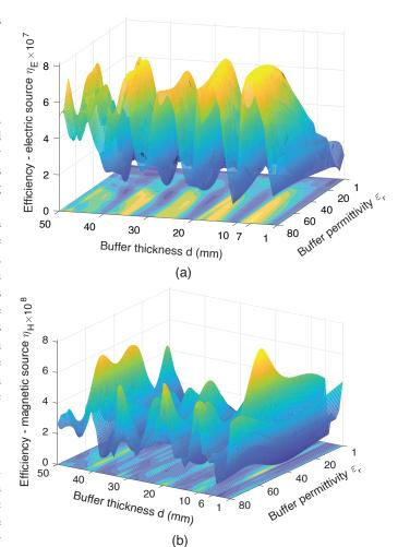
Fig. 2. Wireless power transfer efficiency for the (a) electric and (b) magnetic source as a function of the buffer's thickness d and permittivity  $\varepsilon_r$  at the frequency of 2.45 GHz
