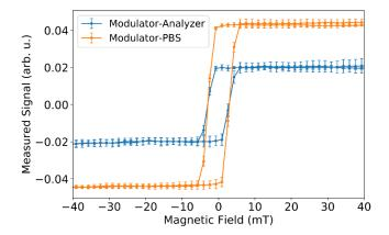
**FIG. 2.** Second harmonic of longitudinal MOKE measurements made with the modulator-analyzer (blue) and the modulator-PBS (orange) setup for a Si/Ta 3/Pt 3/Fe 15/Pt 3 (nm) sample. The error bars correspond to the standard deviation of a set of 4 measurements.
