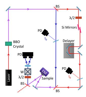
FIG. 3. Experimental time-resolved MOKE setup. The laser is a Titanium-sapphire system with an output wavelength of 800 nm. The beam is frequency-doubled in a BBO crystal. Dichroic beamsplitters are used to separate and recombine the pump (red) and probe (blue) beams. The fluence of the pump beam on the sample is controlled by a half-waveplate coupled with a pair of Si mirrors acting as polarizers. Photodetectors are placed along the paths of the beams to keep track of their intensities.
