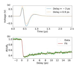
**FIG. 4.** (a) RF output waveforms of the balanced photodetector recorded before (blue solid line) and after (orange dotted line) excitation by the optical pump pulse. The difference between the two waveforms is a consequence of the demagnetization of the sample. (b) Normalized Kerr rotation as a function of time delay for the same sample (green dot). The solid red line shows a bi-exponential fit of the data.
