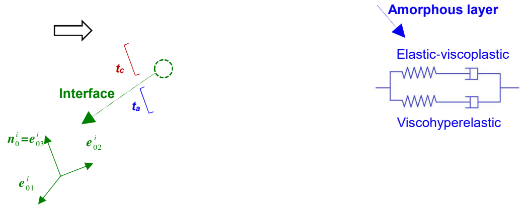
Figure 2. Constitutive representation considering the semi-crystalline medium as an aggregate of randomly distributed two-phase layered composite inclusions. Each inclusion is constituted by a stiff crystalline lamella with an internal elasti-viscoplastic stress and a rubbery amorphous layer with an internal stress including elastic-viscoplastic intermolecular and viscohyperelastic network stresses.
