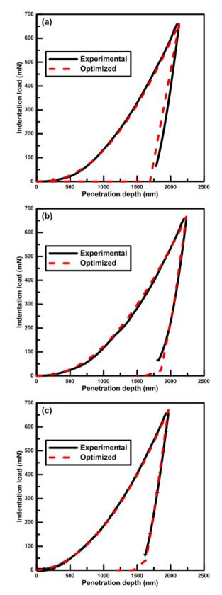
Fig. 6. Comparison of (P-h) curves obtained from experimental data and FE model using the optimized parameters for a substrate bias voltage of: (a) -200 V, (b) -500 V and (c) -700 V.
