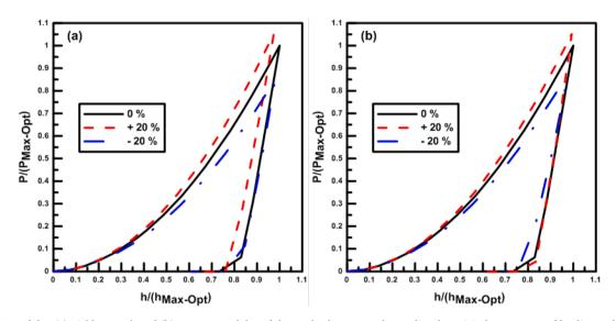
Fig. 8. Effects of the: (a) yield strength and (b) Young's modulus of the steel substrate on the predicted empirical parameters of loading and unloading.
