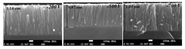
Fig. 1. .Cross-sectional SEM images of the CrN coatings as a function of the substrate bias voltage.
