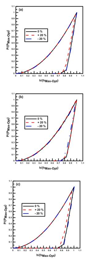
Fig. 7. Effects of the: (a) yield strength, (b)Young's modulus and (c) Strain hardening exponent of CrN coating on the predicted empirical parameters of loading and unloading.
