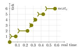
**Figure 4** Graphical representation of an arbitrary clock c and its inverse function  $next_c$ .
