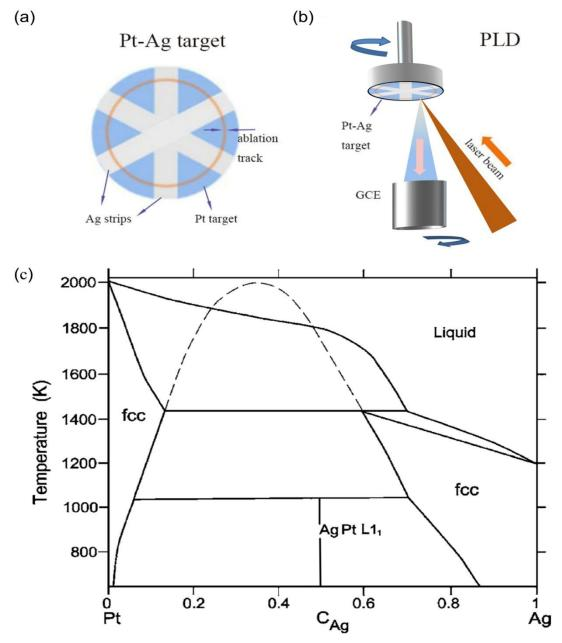
Figure 1. The improved pulsed laser deposition (PLD) method. (a) Pt-Ag Target, the Ag strips distribution on the Pt target, the dotted rings represent the erosion race - track). (b) Schematic illustration of the pulsed laser deposition (PLD) method. (c) Pt-Ag phase diagram based on the assessed experimental phase diagram from Durussel1996 and confirmed by sluiter2006. 40, 41
