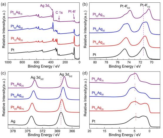
Figure 7. (a) The XPS survey spectra of the as-prepared  $Pt_{75}Ag_{25}$ ,  $Pt_{50}Ag_{50}$  and  $Pt_{25}Ag_{75}$  nanoparticles, (b) High-resolution spectrum of Pt 4f region, (c) High-resolution spectrum of Ag 3d region, (d) Valence band spectrum (VBS) for pure Pt,  $Pt_{75}Ag_{25}$ ,  $Pt_{50}Ag_{50}$  and  $Pt_{25}Ag_{75}$  nanoparticles.
