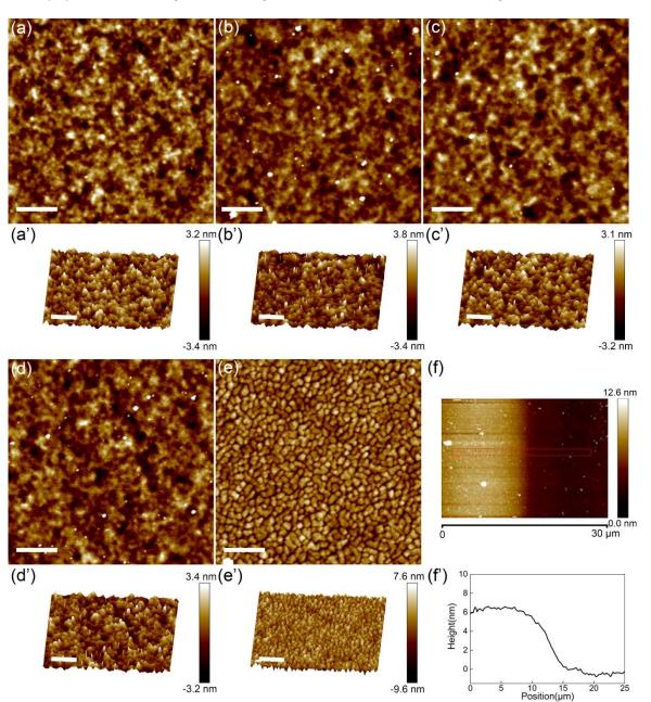
Figure 2. Morphology characterization of as-prepared samples. Tapping-mode AFM images of Pt NP (a), Pt<sub>75</sub>Ag<sub>25</sub> NP (b), Pt<sub>50</sub>Ag<sub>50</sub> NP (c), Pt<sub>25</sub>Ag<sub>75</sub> NP (d), and Ag NP (e). Stereoscopic display of AFM images were corresponding to images of (a'), (b'), (c'), (d') and (e'), respectively. (f) Step of Pt NP sample deposition on the quartz plate. (f') The thickness of pure Pt NP synthesized by PLD for 45 min with 27000 pulses.
