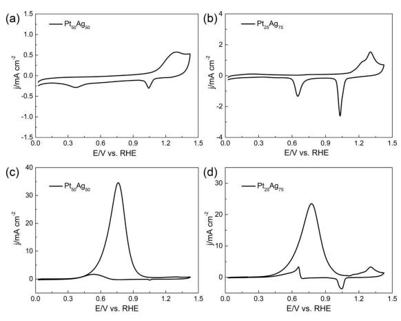
Figure 8. (a, b) Cyclic voltammetry profiles of  $Pt_{50}Ag_{50}$  and  $Pt_{25}Ag_{75}$  nanoparticles in 1 M KOH solution. (c, d) Cyclic voltammetry profiles during methanol oxidation reaction for  $Pt_{50}Ag_{50}$  and  $Pt_{25}Ag_{75}$  nanoparticles in 1 M methanol and 1 M KOH solution. All graphs are at a scan rate of 50 mV s<sup>-1</sup>.
