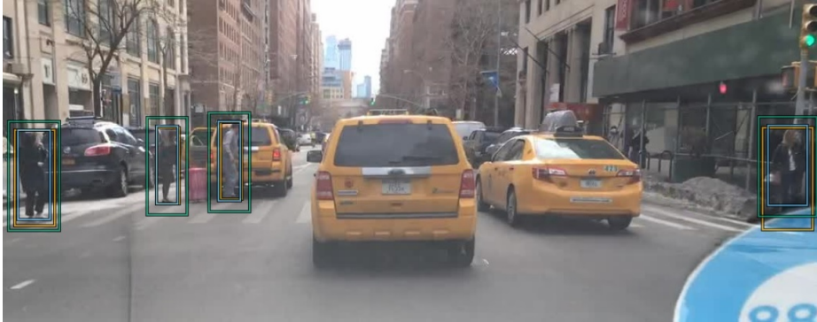
Fig. 1. Conformalization example (box-wise, risk level \alpha = 0.1 ) on a BDD100k image with Ground Truth , Inference and Conformalized boxes.
