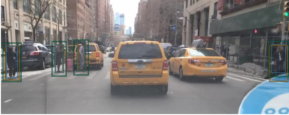
Fig. 1. Conformalization example (box-wise, risk level \alpha = 0.1 ) on a BDD100k image with Ground Truth , Inference and Conformalized boxes.
