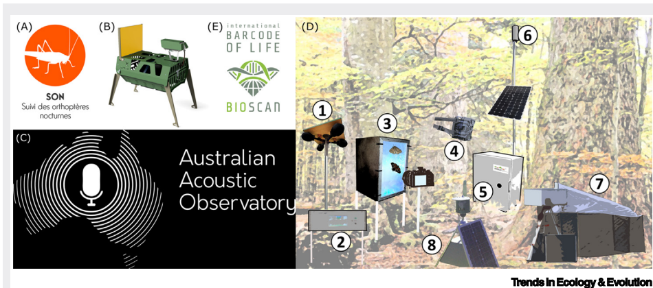
Figure 1. (A) Suivi des Orthoptères Nocturnes, the French nation-wide monitoring scheme for bush crickets. (B) The DIOPSIS (digital identification of photographically sampled insect species) automatic insect monitoring device. (C) The Australian Acoustic Observatory used automatic acoustic sensors to record all environmental sounds. (D) The BIOSCAN project of the International Barcode of Life consortium aims to collect DNA barcodes of 10 million insect specimens and characterise their parasitic, mutualistic, and symbiotic relationships at over 2000 locations worldwide. (E) Illustration of the modular AMMOD (automated multisensor stations for monitoring of species diversity) monitoring station design. (1) Acoustic monitoring. (2) Smellscape (plant volatile organic compounds). (3) Visual monitoring: Moth scanner, (4) Visual monitoring: Wildlife camera trap, (5) Base station, (6) Data transfer and management, (7) Metabarcoding: Automated Malaise trap, (8) Metabarcoding: Automated pollen sampler. Figure draft and design: J. Wolfgang Wägele.
