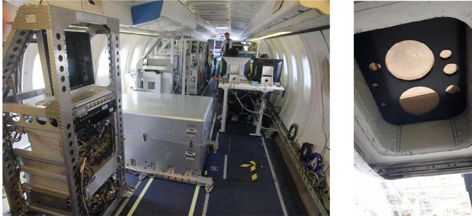
**Fig. 1.** Left: Photograph of the CHARM-F integrated path differential absorption lidar as installed into the French ATR42 aircraft. The instrument consists of two electronics racks and the central optics box containing the lasers, telescopes and detectors. Right: Picture of the optical viewport integrated into the fuselage of the aircraft.
