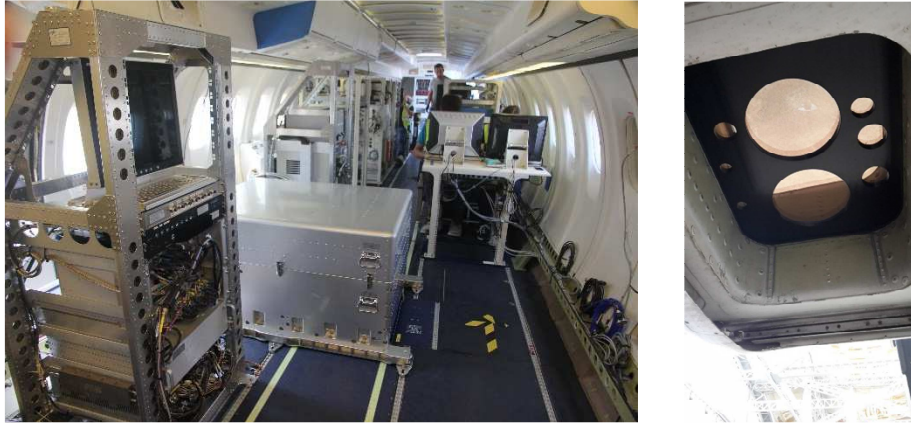
Fig. 1. Left: Photograph of the CHARM-F integrated path differential absorption lidar as installed into the French ATR42 aircraft. The instrument consists of two electronics racks and the central optics box containing the lasers, telescopes and detectors. Right: Picture of the optical viewport integrated into the fuselage of the aircraft.
