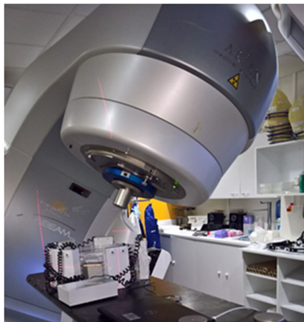
FIGURE 6 Irradiation setup for irradiation with an elliptic field: The LINAC is equipped with a 10-mm stereotactic cone and a 30° gantry is used.
