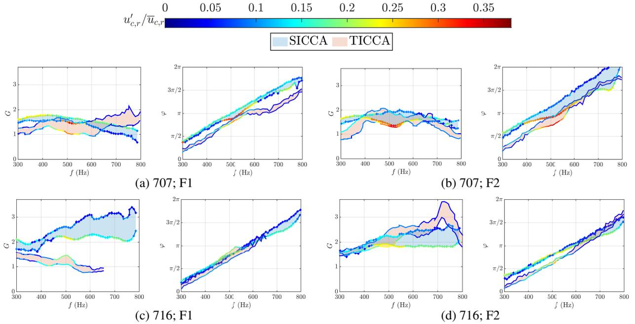
Fig. 8: Comparison of gain  $G$  and phase  $\phi$  of the FDFs measured in the multiple-injector setup TICCA-Spray (solid lines without marker) with co-rotating neighbors and in the single-injector system SICCA-Spray (solid lines with marker) at the two operating points F1 and F2, and for the swirlers 707 and 716. The levels of velocity fluctuations  $u'_{c,r}/\bar{u}_{c,r}$  are indicated by the color levels and the span of the FDF data is represented by the colored bands.
