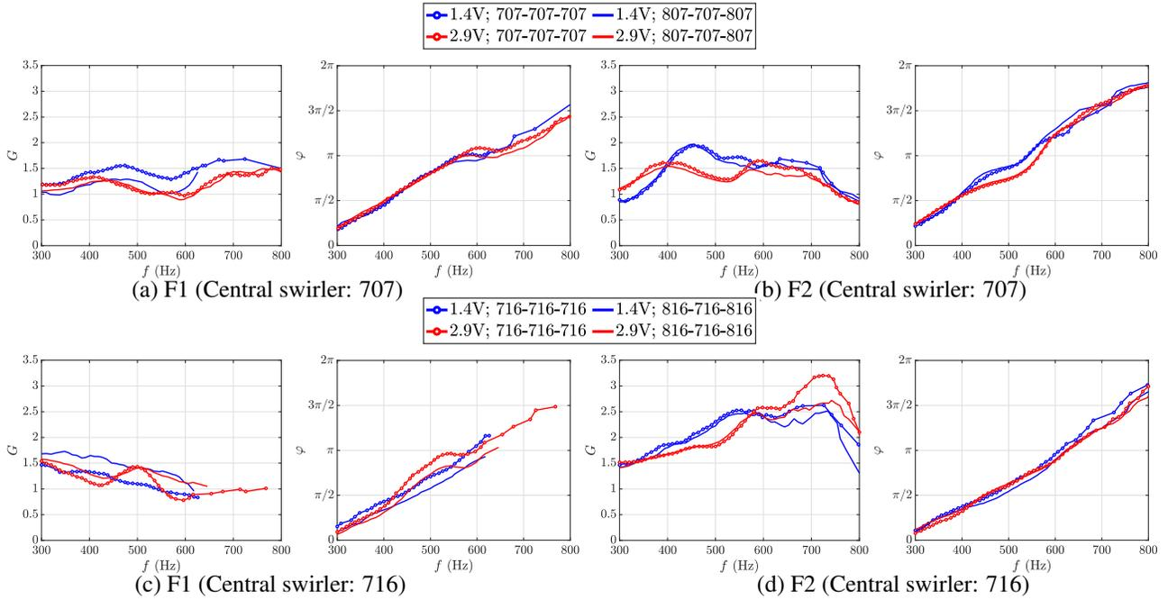
Fig. 7: Influence of neighboring swirlers: gain  $G$  and phase  $\phi$  of the FDF measured in TICCA-Spray with co- (solid lines with marker) and counter-swirl (solid lines without marker) swirler combinations at the two operating points F1 and F2. Results are presented for two amplifier voltage  $V_0 = 1.4\text{ V}$  and  $2.9\text{ V}$  of the driver units.
