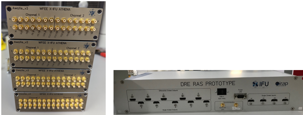
Figure 6. (Left) Part of demonstration model of the Warm Front-End Electronics (WFEE). Each block are SMB connectors for signal output as well as TES bias, MUX SQUID bias and feedback and AMP SQUID flux bias inputs, for two channels (or columns). Those 4 blocks permits to perform 8 column TDM. (Right) Digital Readout Electronics Row Addressing and Synchronisation (DRE RAS) prototype module. There are 5 HDMI outputs (J1 to j5) for differential readout that will be used with WFEE. 5 other HDMI output (J6 to J10) are used in the actual single-ended readout electronics, allowing to test until 17 pixels in a column.
