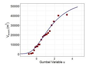
Fig. 2. Claret's Frequency - Magnitude curve obtained after the adjustment of recorded debris flow events using generalized Pareto distribution (Adapted from (Morel et al., 2022)).
