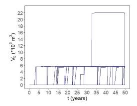
Fig. 7. Deterioration trajectories showing the filling of the Claret's debris basin over time for the 100 generated scenarios - New design.
