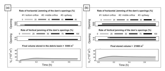
Fig. 3. Results obtained from the physics-based model showing the variation of the dam's openings jamming rate and the volume stored in the basin over time: (a) event 1 in scenario 1 and (b) event 2 in scenario 1 - Initial design.
