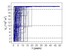
Fig. 4. Deterioration trajectories showing the filling of the Claret's debris basin over time for the 100 generated scenarios - Initial design. Dashed lines are the chosen thresholds corresponding to the proposed condition at which maintenance operations are carried out:  $V_b^i = 0$ , 2, 200, 10, 000 and 20, 000  $m^3$ .
