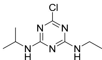
**Figure 1.** Atrazine (2-chloro-4-ethylamino-6-isopropylamino-1,3,5-triazine).
