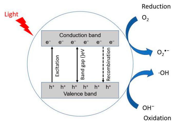
**Figure 2.** Schematic representation of mechanism of photocatalysis.
