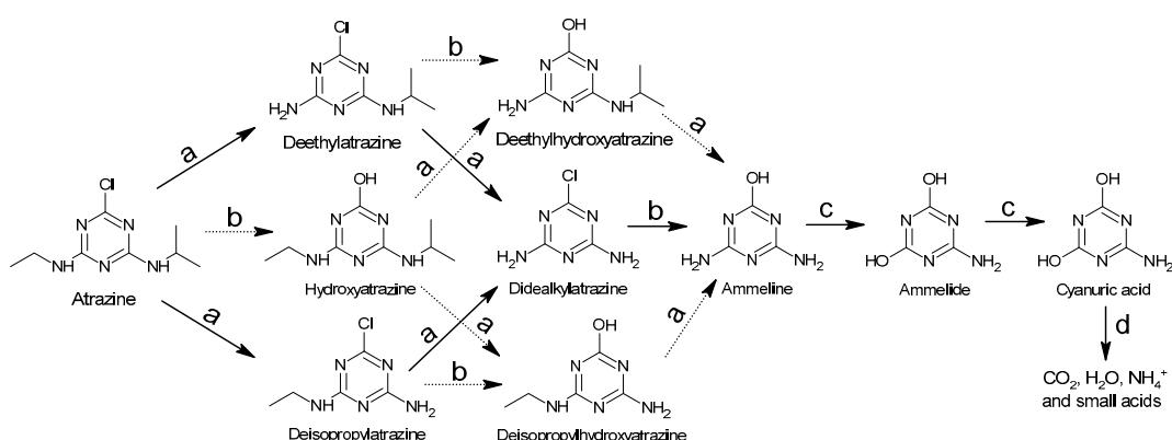
**Figure 4.** General involved degradation mechanisms of atrazine: (a) dealkylation of the amino groups; (b) dechlorination and hydroxylation of the s-triazine ring; (c) oxidation of the amino groups and deamination; (d) the opening of the s-triazine ring.
