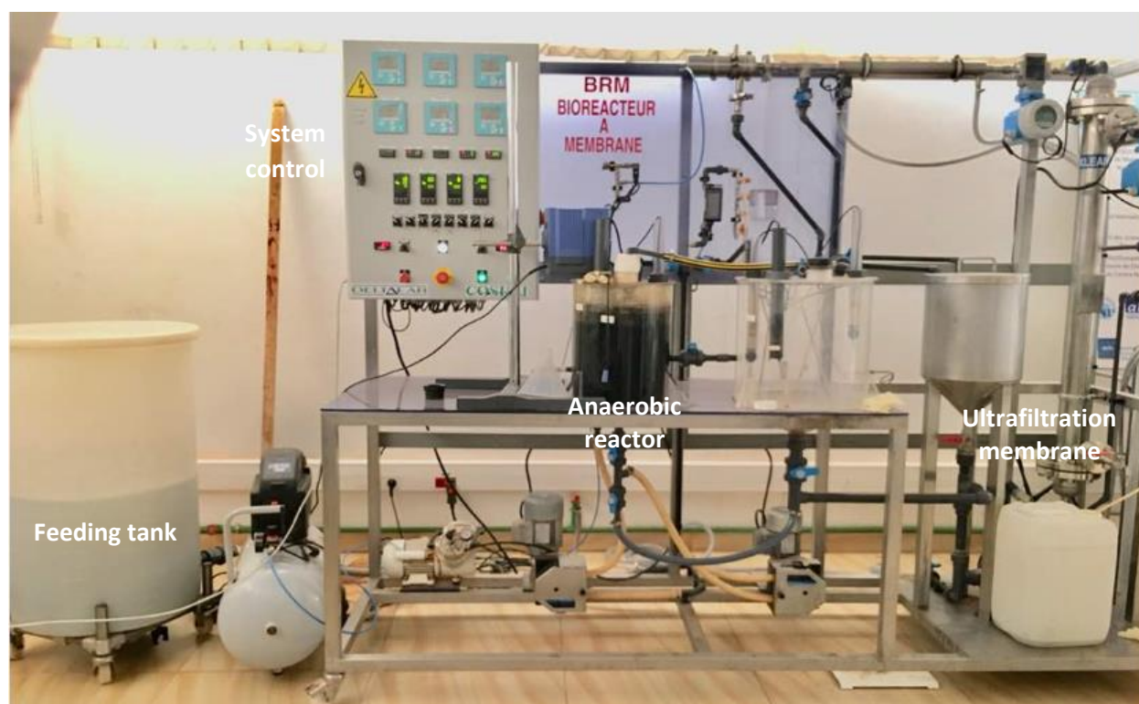
Figure 1: AnMBR pilot using for the beverage wastewater treatment
