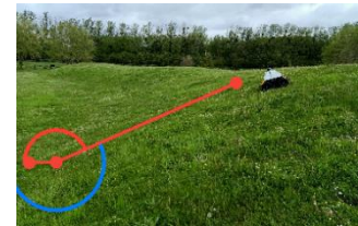
Figure 12 UGV i on grass 24° slope
