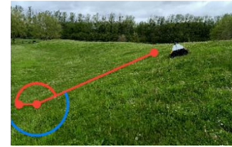
Figure 12 UGV i on grass 24° slope
