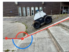
Figure 9 UGVi on tarmac 25° slope
