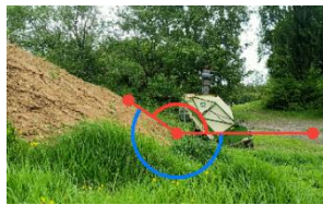
Figure 7 UGVi climbing test 35° slope on wet grass
