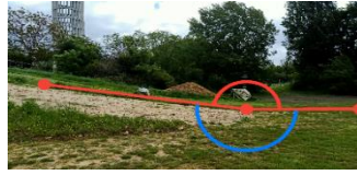
Figure 11 UGV i on grass 18.5° slope
