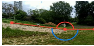
Figure 11 UGV i on grass 18.5° slope
