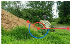
Figure 7 UGVi climbing test 35° slope on wet grass
