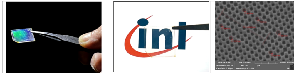
Fig. 10. Views of samples at grazing incidence (on the left, the green color can be related to the diffraction of the Bloch mode in S polarization that exists at large wavelengths for such patterns and that is partly visible in Fig. 7 and Fig. 11) and under normal incidence (in the middle, the sample is transparent). SEM image of one the fabricated sample (on the right).
