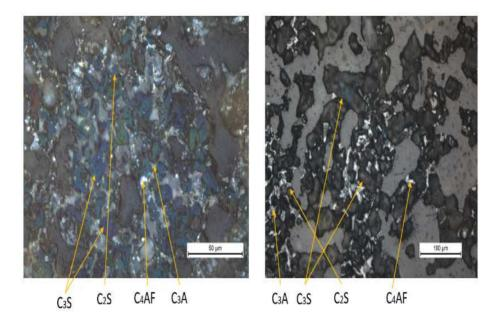
**Fig. 8** Observation by optical microscope on the polished section of CP 97 TM (left) and CP 97 (right) clinker
