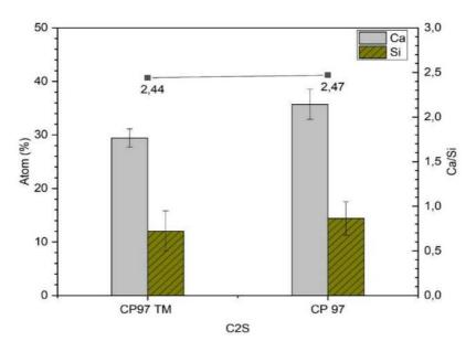
395 Fig. 10 Chemical composition and the ratio of major elements of C<sub>2</sub>S phase
