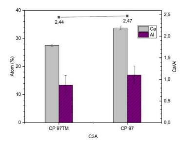
411 Fig. 11 Chemical composition and the ratio of the major elements of C<sub>3</sub>A phase
