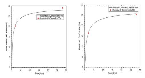
Fig. 21 CH/initial cement mass ratio of OPC 97 TM (left) and OPC 97 (right) cement paste 584
