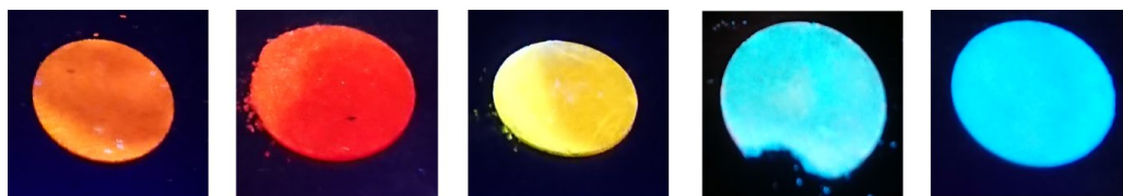
Figure 10. Emission color of KBr pellets doped with 2% of chromophores (from left to right: 9b , 10a , 10b , 11a , 11b ). The picture was taken in the dark upon irradiation with a handheld UV lamp ( \lambda_{\text{exc}} = 366 \text{ nm} ).
