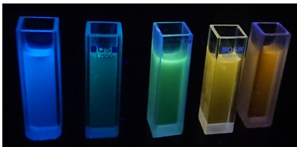
Figure 6. Fluorescence color change experienced by 11a in various solvents (from left to right: n -heptane, toluene, 1,4-dioxane, \text{CHCl}_3 , DCM). The picture was taken in the dark upon irradiation with a handheld UV lamp ( \lambda_{\text{em}} = 366 nm).
