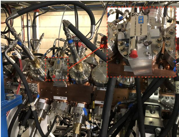
Figure 3: Detector installed on the RFQ flange.
