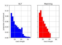
Fig. 3: Histogram that represents the lengths of tracks *i.e.* the number of keyframes on which a landmark is detected for a matching based VO and a tracking based VO.
