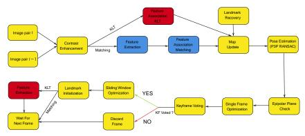
Fig. 2: Pipeline of both matching based and tracking based Visual Odometry. Steps relative to tracking design are in red, whereas boxes referring to matching design are in blue.
