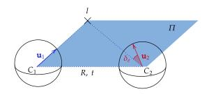
Fig. 1: Illustration of the epipolar angular error.  $\prod$  is the epipolar plane,  $\{C_1, C_2\}$  are the optical centers of the two views and  $\{\mathbf{u_1}, \mathbf{u_2}\}$  are the two bearing vectors of landmark l observation.
