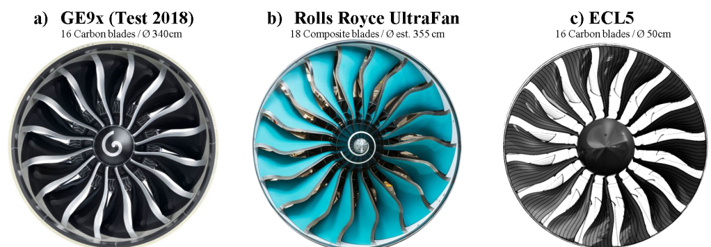
Figure 2. Modern industrial low-speed composite fans and Open-Test-Case ECL5/CATANA (CAD)
