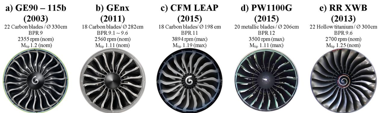
Figure 1. Selection of established modern (Ultra)-High-Bypass-Ratio Engines
