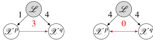
Figure 8: How TCDF deals with hidden confounders. A red edge (left) indicates a wrong causal relation discovered by TCDF, whereas a red double edge (right) indicates that a true causal relation is discovered. Numbers correspond to delays.
