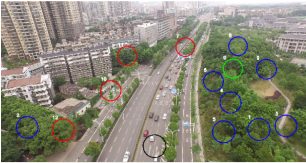
Fig. 5: Example outputs for Emergency Landing. Circles are candidates identified by the main model, colors indicate runtime monitor status. The default action consists in opening a parachute without moving. Source: [11].
