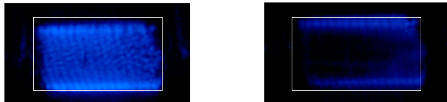
Figure 1. Typical discharge appearance with partial discharging and different \beta percentages (white frame showing the limits of the reactor).
