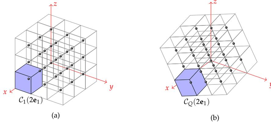
Fig. 1: (a) illustrates a set of points of  $\mathbb{Z}^3$  as black points, whose associated digitization cells (voxel) are represented by wireframed cubes. The cube colored in blue is the digitization cell of  $2\mathbf{e}_1$ , i.e.,  $C_1(2\mathbf{e}_1)$ . (b) shows the rotated points and digitization cells by a geometric algebra rotation  $Q$ , where the cube colored in blue represents  $C_Q(2\mathbf{e}_1)$ .
