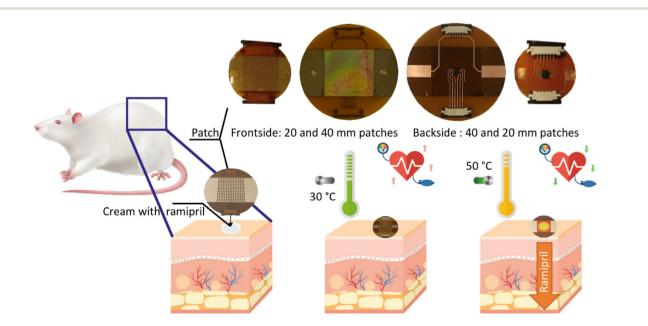
Fig. 1 In vivo model for electrothermal ramipril delivery. Enhanced ramipril permeation upon combination of nano-engineered heating elements with a transdermal vehicle, Pentravan® loaded with ramipril (10%).
