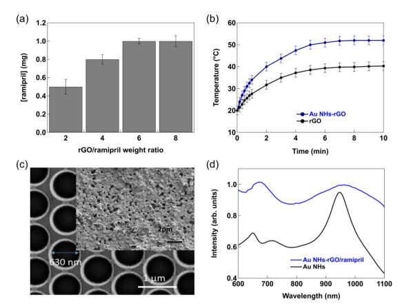
**Fig. 2** Ramipril loading onto rGO-coated nano-heating elements. (a) Ramipril (1 mg) loading capacity of rGO as a function of rGO/drug ratio. (b) Photothermal heating curves of water using rGO directly deposited on Kapton or on a nano-heater in the form of Au NHs. (c) SEM image of Au NHs without and upon coating with rGO/ramipril (inset). (d) UV-Vis absorption spectra of Au NHs and Au NHs-rGO/ramipril in air.
