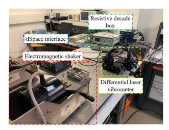
Fig. 4. Experimental testbench.
