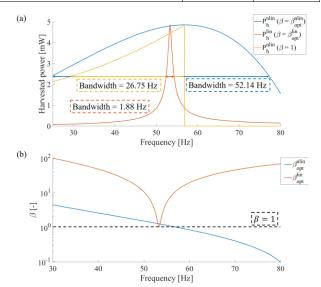
Fig. 3. (a) harvested power and (b) optimal electrical damping for the linear (orange) and the non-linear (blue and yellow) model.
