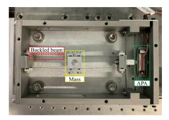
Fig. 1. Bistable piezoelectric energy harvester.
