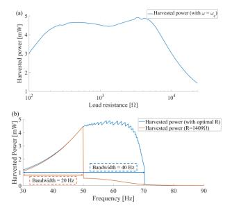
Fig. 7. (a) harvested power as a function of the load resistance for the critical frequency, (b) maximum harvested power (blue line) and harvested power for the maximum electrical damping (orange line) as a function of the frequency.
