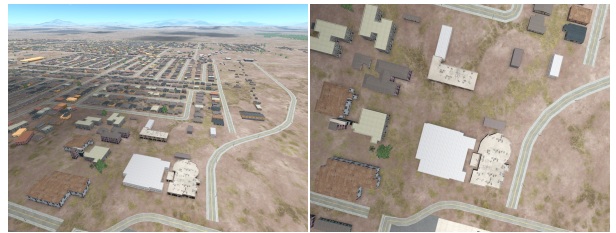
Figure 9: Camera oriented to the front (left) and to the nadir on the same scene (right). The optimal pitch depends on the application.
