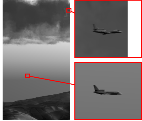
Figure 14: Synthetic IR images simulated using a physics based rendering engine.
