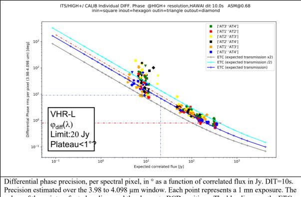
Precision estimated over the 3.98 to 4.098 µm window. Each point represents a 1 mn exposure. The colors of the points refer to baselines and the shapes to BCD positions. The blue lines are the ETC predictions. The red dash-dotted line is a median ETC update fitted through the data. A precision of 4°/spectral channel is equivalent to 9°/spectral pixel (~5 pixels/channel). This equivalent to a coherent flux SNR=10 per spectral channel. This is achieved for a 20 Jy source.
