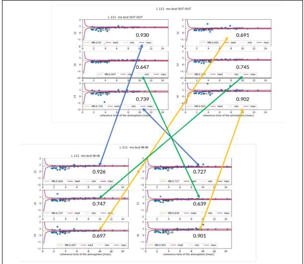
Figure. 14.1: Broadband L-band instrumental visibility plotted as a function of the coherence time for the two BCD configurations OUT-OUT and IN-IN. The average visibility level for every baseline is indicated in bold font. This average visibility has been estimated from a large number of observations over more than 18 months
