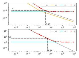
From top to bottom: the visibility, the closure phase and the differential phase errors as a function of flux in Jy. The plots on the left are those of the fundemental noise. The plots on the right are those of the global error, in red, and its components: -the fundamental noise in grey -the error due to the seeing variation, in cyan -the error related to a wrong background correction, when applicable, in orange
