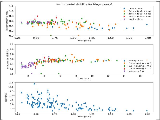
Figure 2.5: An example of the variation of instrument visibility with seeing conditions. In L band with DIT=75 ms. Note that we are very strongly dominated by the sensitivity to Tau0. After Tau0~5 ms, the sensitivity to seeing is strongly reduced. For Tau0 lower than 3 ms, we can have a reduction in instrumental contrast by a factor 2.
