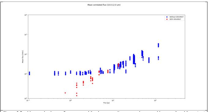
Figure 2.7a: Measured coherent flux, corrected for the source diameter and averaged between 8 and 9  $\mu$ m (top) and 10-12  $\mu$ m (bottom), as a function of the Wise W3 N band flux of the calibrator. The blue dots are for MATISSE alone observations N band coherent flux integration with piston correction from the N band itself (coherent algo=2). The red dots are for N band coherent integration using GRA4MAT
