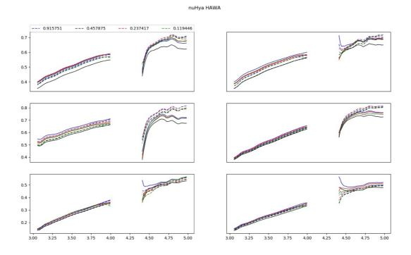
Figure 13.2: The six L&M band Hawaii2RG visibilities obtained on nu Hya for 4 different chopping frequencies, chopping data refer to the dashed lines: 0.92 (blue), 0.46 (green), 0.24 (red) and 0.12
