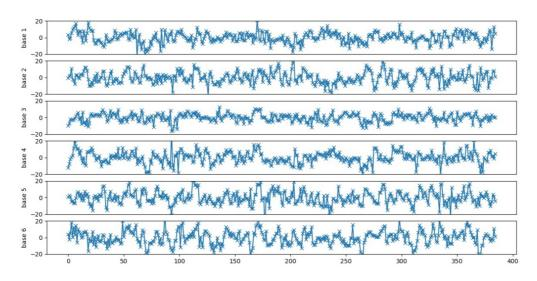
*Figure 4.1.4: OPD residuals for the 6 baselines during a 1mn observation using the internal MATISSE fringe sensing.*
