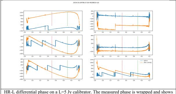
HR-L differential phase on a L=5 Jy calibrator. The measured phase is wrapped and shows  $2\pi$  jumps. We use an unwrapping python function before applying the ETC procedure. We see here that the unwrapping can partially fail or need to be iterated. The user should be aware of this phase wrapping problem, even if we plan to correct this in the DRS. This problem is not critical for local continuum-line-continuum measurements.
