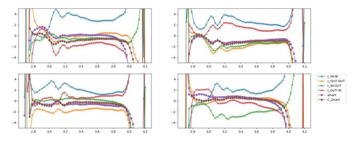
Figure 8.4a. Calibration of the closure phase in the L band with one calibrator for the four BCD positions (c\_IN-IN,c\_OUT-OUT,c\_IN-OUT,c\_OUT-IN). with the BCD alone (purple line; smart) and with both the BCD and calibrator (brown; C smart)
