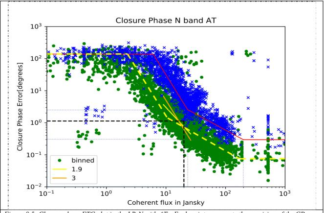
Figure 8.5: Closure phase ETC plot in the LR-N with ATs. Each point represents the precision of the CP per spectral channel and per exposure between 8 and 9  $\mu$ m. The blue crosses are for data reduced without a priori binning and the blue points for binned data. The over plotted lines are attempts to fit the measurement error. The best result is obtained with an  $f^1$  fit for bright targets and  $f^3$  fit for fainter targets.
