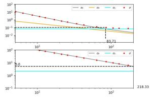
From top to bottom: the visibility, the closure phase and the differential phase errors as a function of flux in Jy. The plots on the left are those of the fundemental noise. The plots on the right are those of the global error, in red, and its components: -the fundamental noise in grey -the error due to the seeing variation, in cyan -the error related to a wrong background correction, when applicable, in orange
