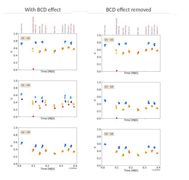
Figure 14.2: Plot of the broadband L-band transfer function (between 3.1 and 3.9 um) for the night of Feb 23, 2022, with the effect of the BCD (Left) and with the BCD effect removed by the chromatic correction factor applied to the IN-IN visibilities (Right). The dots and squares correspond to the OUT-OUT and IN-IN configurations, respectively. Blue (dark and light) and red/orange colors correspond to calibrator and science targets.
