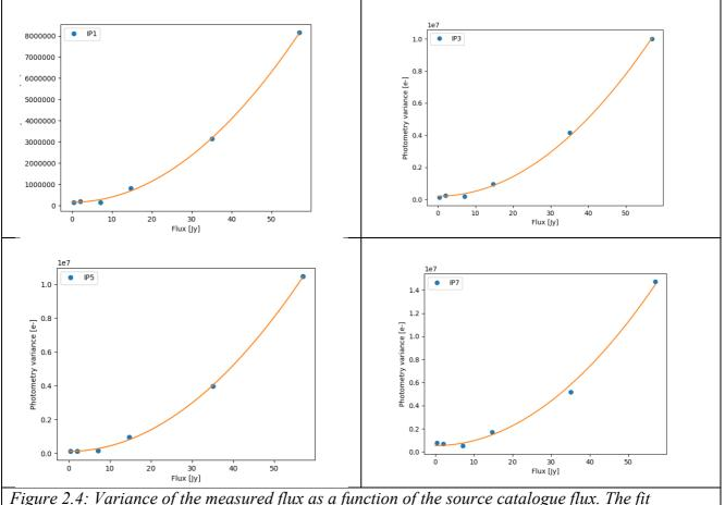
Figure 2.4: Variance of the measured flux as a function of the source catalogue flux. The fit contains a constant term that is the source independent photometric noise, a term proportional to the source flux, that is the source photon noise and a term proportional to the square of the source flux that is the residual fraction of the source in the sky image.
