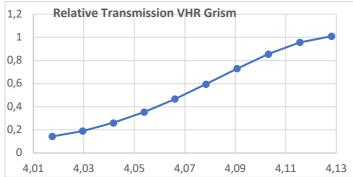
Figure A: Relative transmission of the VHR grism in L band. At 4.052 $\mu$ m (Br $\alpha$ ) the transmission is 35% of the one at 4.128 $\mu$ m.
