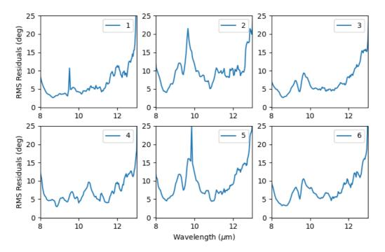
*Figure 15.4 RMS of residuals when calibrating zero phase sources in N with a single nearby calibrator*
