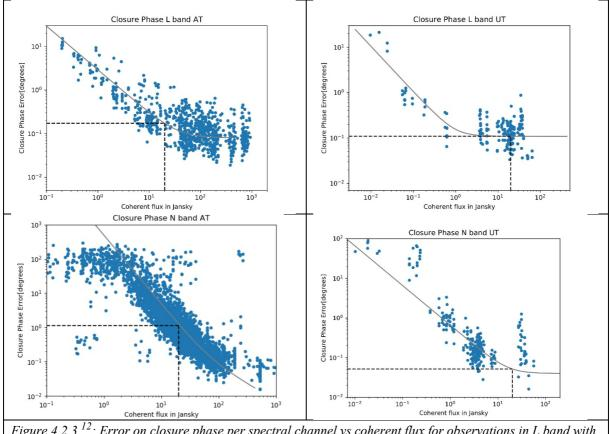
Figure 4.2.3 <sup>12</sup>: Error on closure phase per spectral channel vs coherent flux for observations in L band with ATs (upper left), in L band with UTs (upper right), in N band with ATs (bottom left) and in N band with UTs (bottom right).
