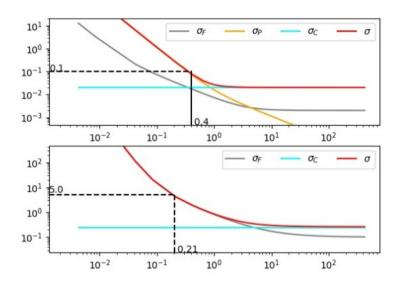
From top to bottom: the visibility, the closure phase and the differential phase errors as a function of flux in Jy. The plots on the left are those of the fundemental noise. The plots on the right are those of the global error, in red, and its components: -the fundamental noise in grey -the error due to the seeing variation, in cyan -the error related to a wrong background correction, when applicable, in orange
