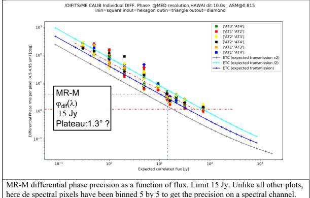
Then the specification is directly 4° per spectral channel that yields a limit M~15 Jy.
