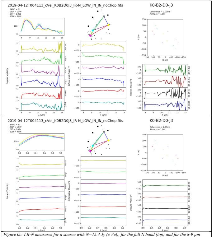
Figure 0c: LR-N measures for a source with N=15.4 Jy (c Vel), for the full N band (top) and for the 8-9  $\mu$ m window (bottom). The limits in LR-N, at 8.5  $\mu$ m, are 16.8 Jy for absolute visibility, 9.4 Jy for Closure phase and 6 Jy for Differential phase.
