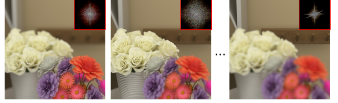
Fig. 2. Disparity space and corresponding Fourier disparity layer representation. The magnitude spectrum of each layer is shown in the red box.
