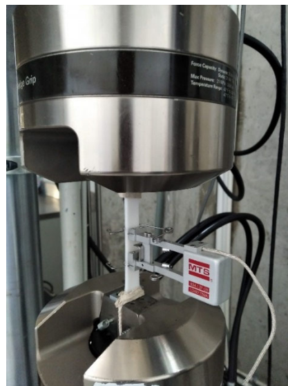
Figure 3. Experimental setup of a tensile specimen.
