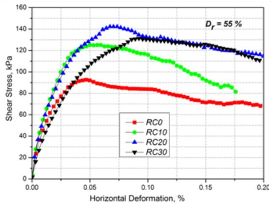
Figure 6. Shear stress variation curves for different relative density: ( $D_r=95\%$ ) and ( $D_r=55\%$ )
