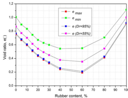
Figure 3. Variation of the maximum and minimum void ratios versus rubber content
