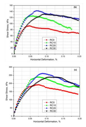
Figure 4.Shear stress variation curves for different rubber contents under a normal stress of: 100kPa (a), 200kPa (b) and 400 kPa (c) (Dr = 55 %)
