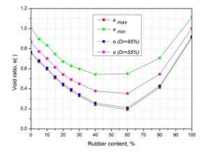
Figure 3. Variation of the maximum and minimum void ratiosversus rubbers content
