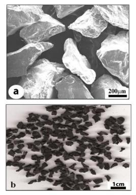
Figure 2.Microscopic view of the Hostun sand (a) and aggregates rubber with 2mm<D<sub>GR</sub><5mm (b).
