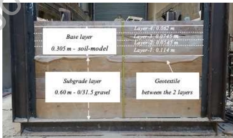
Figure 5: The different layers of the road platform
