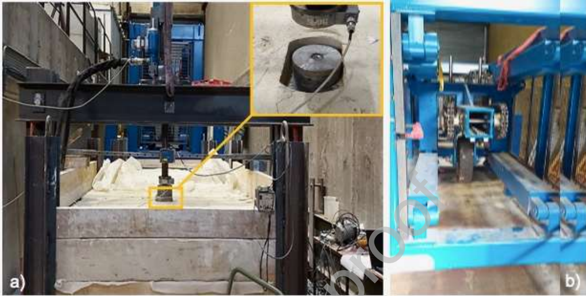
Figure 8: (a) Global view of the cyclic plate loading test device: support beam, hydraulic jack and plate, (b) Traffic load simulation on the road platform
