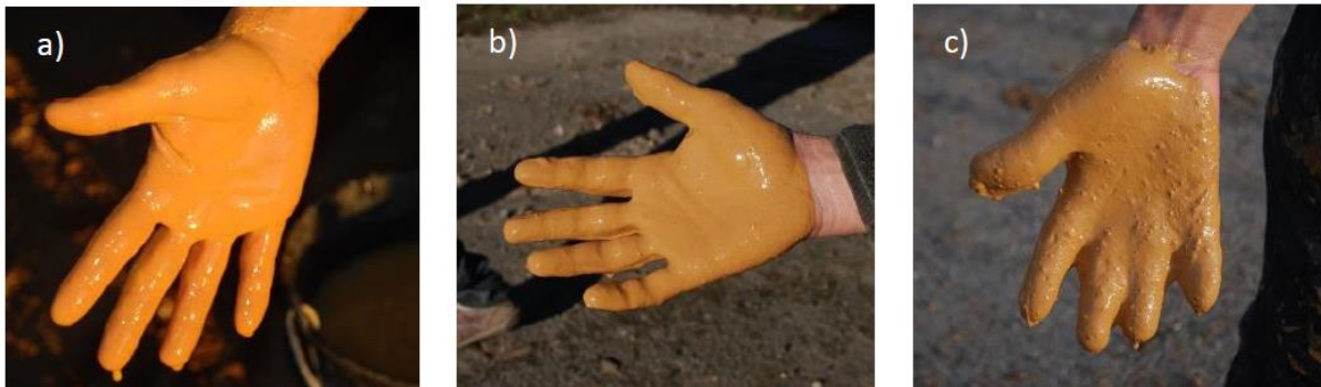
757 758 Figure A.2: Glove test carried out on site. a) the earth slip is too fluid, the hand appears through; 759 formulation of the earth slip is correct when it forms a perfect glove on the hand, without transparency of
