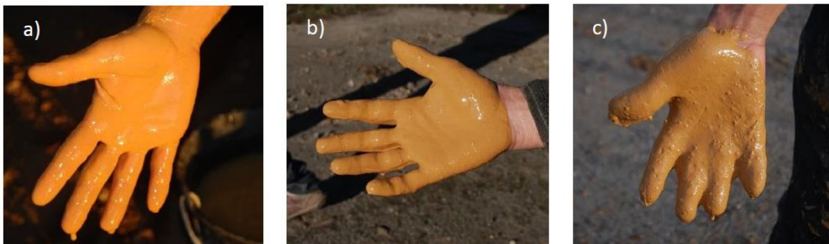
757 758 Figure A.2: Glove test carried out on site. a) the earth slip is too fluid, the hand appears through; 759 formulation of the earth slip is correct when it forms a perfect glove on the hand, without transparency of
