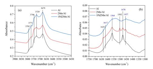
**Figure 6.** FTIR spectra of catalysts after activation at 450 °C under vacuum. (**a**): *v*(OH) vibration; (**b**): carbonate wavenumber zone.
