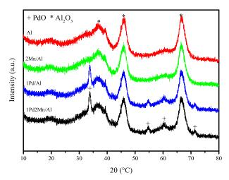
Figure 2. XRD patterns of the catalysts.
