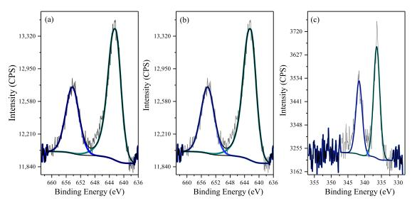
Figure 5. XPS profiles of Mn 2p of (a) 2Mn/Al and (b) 1Pd2Mn/Al and (c) Pd 3d of 1Pd2Mn/Al.
