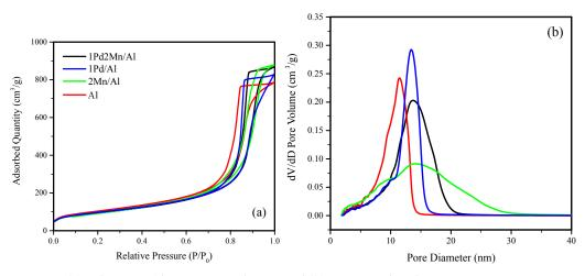
Figure 1. (a) Adsorption/desorption isotherms and (b) pore size distribution.
