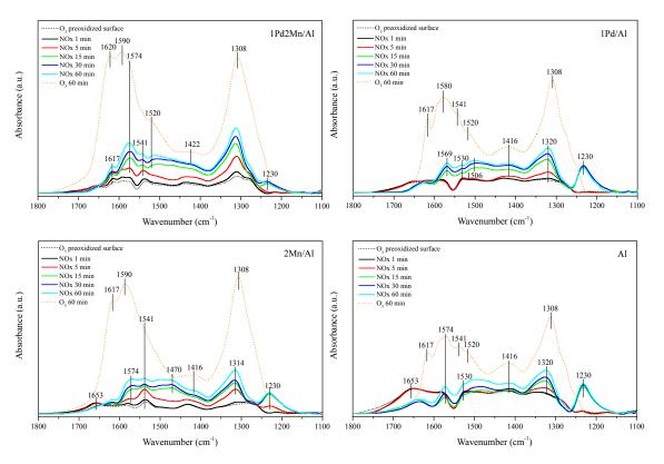
**Figure 10.**  $O_3$  adsorption for 60 min (pre-oxidation of the catalyst) prior to NO/O<sub>2</sub> adsorption for 120 min prior to a second O<sub>3</sub> adsorption for 60 min on different catalysts that are pre-oxidized by ozone (Sequence 2).
