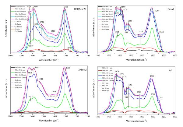
**Figure 11.**  $O_3$  and NOx co-adsorption for 120 min prior to ozone purge for 60 min (Sequence 3) on different catalysts.
