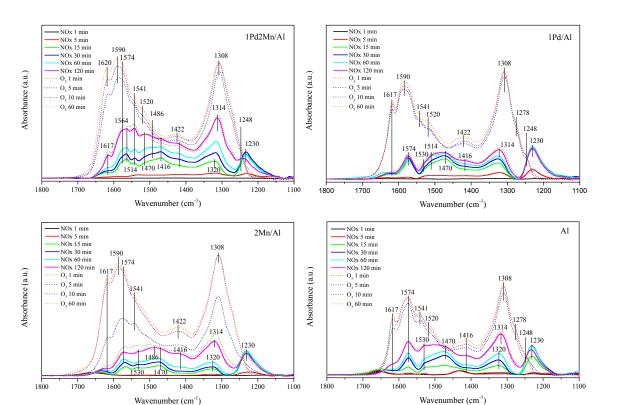
**Figure 8.** NO/O<sub>2</sub> adsorption at 40 °C for 120 min prior to  $O_3$  adsorption for 60 min (Sequence 1) on different catalysts.
