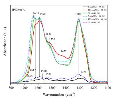
**Figure 13.** Comparison between Sequence 3 and Sequence 4 for 5 and 120 min of NOx adsorption before (solid line) and after (dash line) O<sub>3</sub> adsorption, followed in both case by 60 min of O<sub>3</sub> adsorption.
