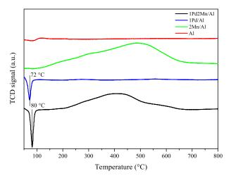
**Figure 4.** H<sub>2</sub>-TPR profiles of all catalyst samples.
