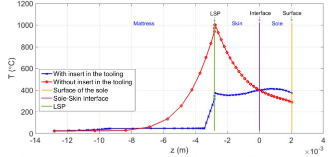
Fig. 8: Temperature at the center from the surface of the sole to the mattress of the configuration 3 with and without insert in the tooling at 10 s
