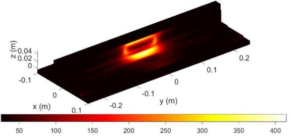
Fig. 7: Thermal image of the 3D model obtained at 10 s heating of the Configuration 3
