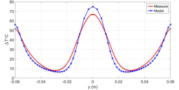
Fig. 5:  $\Delta T$ (°C) at  $x = 0$  of the measurement and the model
