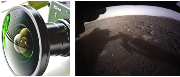
Figure 6: Left : Fisheye lens. Photo: Wikipedia. Right : First high-resolution color image sent by Hazard Cameras (Hazcams) of NASA’s Perseverance Mars vehicle after its landing on February 18, 2021. Distortion effects are in particular visible through the curved horizon line. Photo: NASA / JPL-Caltech.
