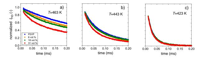
**Figure 5**: Normalized  $I_{FID}$  signals for the net P2VP and the nanocomposites loaded with 6, 18 and 31 vol.% in silica measured at a) 463 K, b) 443 K and c) 423 K. Intensity normalization is performed by using the zero-time limit from the IFL model fit as shown in Figure 6.
