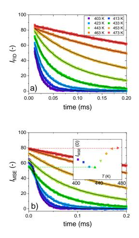
**Figure 3**: a) Raw  $I_{FID}(t)$  signal measured from the neat P2VP between 403 and 473 K. b) Analogous data for  $I_{MSE}(t)$ . Solid lines represent joint fits to the data  $(I_{FID}, I_{MSE})$  for each temperature with the AW function (Equation 3) considering a log-normal distribution of  $\tau_c$  (see text). The inset shows the expected non-monotonic variation of the MSE-FID signal at short time with the temperature (see refs. <sup>19,20</sup>).
