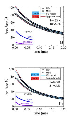
**Figure 6**:  $I_{FID}$  and  $I_{MSE}$  raw signals measured at T=453 K. Light blue and red solid lines stand respectively for the IFL and the  $T_g$  gradient models. a) Nanocomposite loaded with 18 vol.% and b) 31 vol.%. The insets represent the FID contributions of the bulk P2VP and the interfacial layer from the IFL model.
