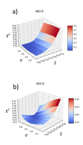
**Figure 8**: Fitting quality ( $\chi^2$ ) as a function of *S* and  $\sigma$  representing respectively the anisotropy of the segmental motion and the breadth of the segmental relaxation time distribution in the IFL model. Fits are performed on data measured on the nanocomposite loaded with 31 vol.% in silica at a) 463 K and b) 443 K.
