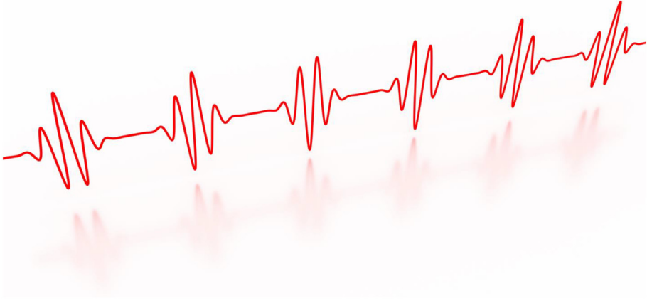
FIG. 3.1 – Schematic illustration of the electric-field structure of a linearly polarized ultrashort pulse train. © MS, Martin Saraceno, 2021.
