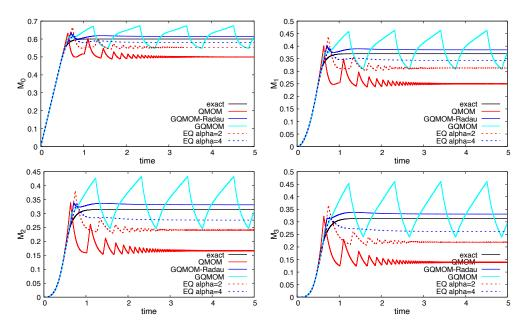
Figure 11: Comparison of different closures for test case with nucleation, growth and filtration: moments of order 0, 1, 2 and 3 for the analytical solution, QMOM with four moments (i.e.,  $M_3$ ), gamma–GQMOM and gamma–GQMOM–Radau with four moments and entropic quadrature (EQ) with multiplicative factor  $\alpha = 2$  and  $\alpha = 4$ .
