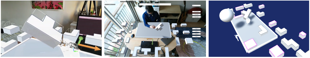
Fig. 2. Remote-view configurations tested by our first study: HEADSET VIEW (left), EXTERNAL VIEW (middle) and VIRTUAL VIEW (right). A remote participant gives oral instructions to the AR user on how to position 3D shapes on a virtual support.
